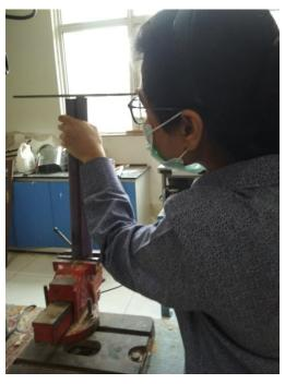
2. Modification of the base required. Switches the footrest to be made from a cross section of a PVC pipe. Sketched grooves where cutting, drilling, filing was required. Cut the primary grooves on either side of the heel end of the pipe till the approximate middle. Drilled the holes where the rods were to be attached. Filed the edges and smoothed the entire footrest.
